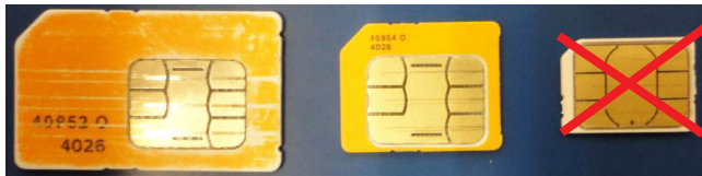
Standard (Mini) SIM card 15 x 25 mm
